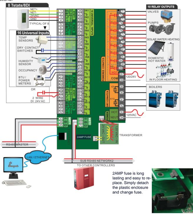
4-wire tstat(over 485) or 2-wire DI(24VAC) can be adjusted by each jumper as right the diagram displayed.
