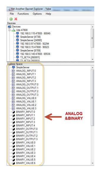
Step4.In the "Address Space" tab, click the "ANALOG\_VALUE", it will show the information of "log ANALOG\_VALUE" in the BacnetProperty tab. And it 's the same with "ANALOG\_OUTPUT" and other items.
