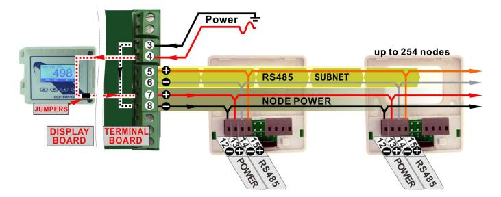
other masters in the system as above, but the transducer analog signals are not available now, instead we now have a second RS485 port which can be used to poll a subnetwork of remote RS485 CO2 sensors. The unit acts as a modbus slave on the main network and a master on the subnetwork. Power to the nodes can be run from Pins 5 and 6 along with the RS485 cable, in this case power makes its way through the display board and jumpers as shown with the dotted lines. If there are more than five
