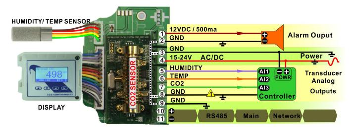
The next diagram shows the wiring connection in 'Master' mode where the device operates as a gateway to a subnetwork of slave sensors. This is a special mode of operation and most users needn't to be concerned about the details of this feature. The main RS485 network is still available on pins 10 and 11 for connecting to
