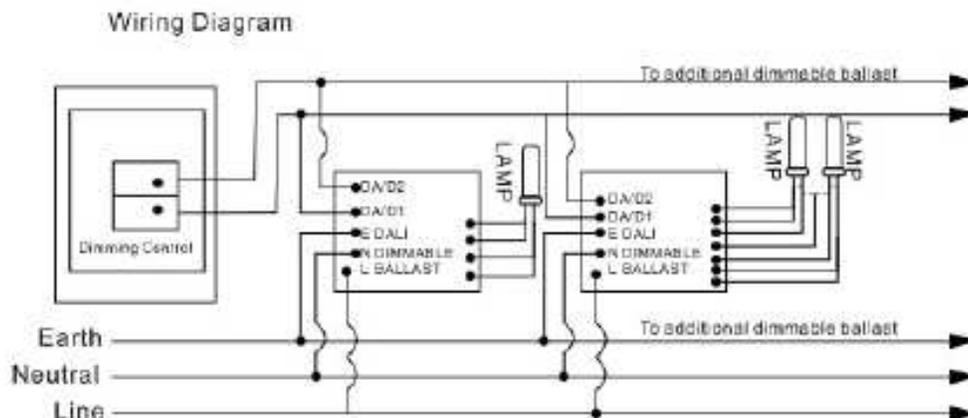
Ballast has plug in wire trap connectors.
