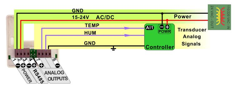
The next diagram shows the HUM Node working in the RS485 network, the node quantity can be 255. A group of sensors distributed through the building can cooperate friendly through net. The RS485 network is available for transmitting the same values digitally to other controllers.
