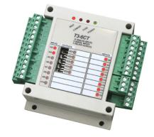
T3-6CT: 10 Universal Inputs 6 AC Current Inputs (6 CTs) 5 Relay Outputs
