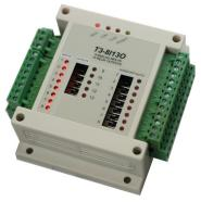
T3-8I13O: 8 Universal Inputs 13 relay outputs
