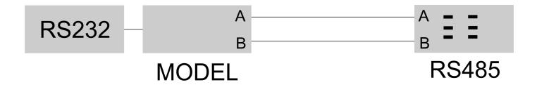
Two point-to-multipoint asynchronous half duplex communication
