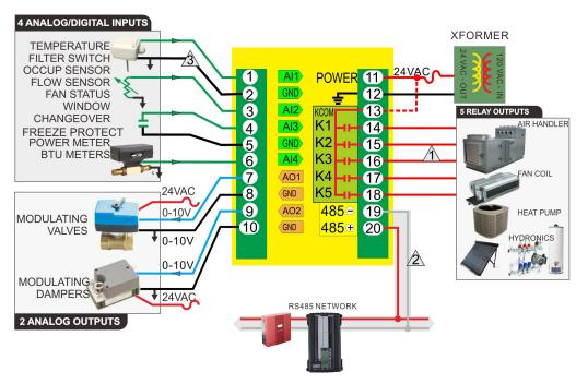
Relay outputs: 24VAC@1amp max, 3 amp combined max for all 5 outputs
