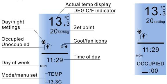
The LCD panel displays a wide variety of functions that Tstat7 thermostat can do to create a comfort level like no other. Be able to automatically adjust the heat, cool, and fan modes to which ever temperature you desire; day or night. You can also program the thermostat to operate at a lower level when the room or building is unoccupied, saving energy and costs on your electric bill, what's more, the earth will become more and more beautiful and ecological.
