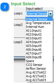
For the PID feedback you can select from many options such as the average of some sensors, any of the 8 external sensors or the internal humidity or C02 sensor if it has one.
