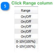
Click the Range column to see many options available for the range setting such as PWM and floating three wire control for modulating actuators using two relay outputs.
