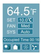
2.In normal mode, press both and at the same time, and hold for several seconds, this will switch to the menu mode. Press or to scroll through the menu options such as 'Add', 'CAL', 'bAU', 'UNI TS' and many others. To change the values at a particular menu, press or the value will be stored automatically.
