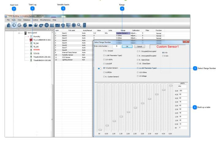
As an example of a custom sensor, here we have built up a table for a custom sensor operating from 0 to 5V over the range of 0-100psi.
