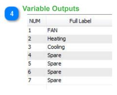
Click to give each output a name and a range, in the case of the fan the outputs are on-off and the valves are modulating 0-10V = 0-100% which are the default ranges already.
