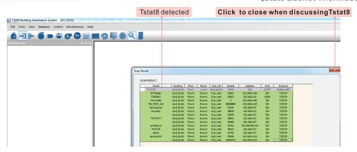
4. Click Tstat8 log, then click , this will display all of the Tstat8 inputs. Change the name of the input and range that fits the application.
