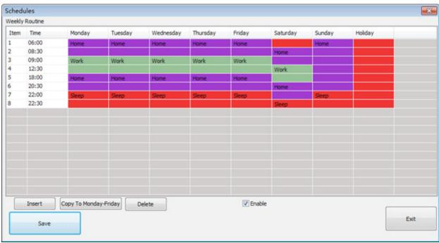
So on Saturday, when time is between 8:30 to 12:30, unit will work on home mode; when time is between 12:30 to 20:30, unit will work on work mode; when time is between 20:00 to 22:30, unit will work on home mode; when time is between 22:30 to Sunday 6:00, unit will work on sleep mode.
